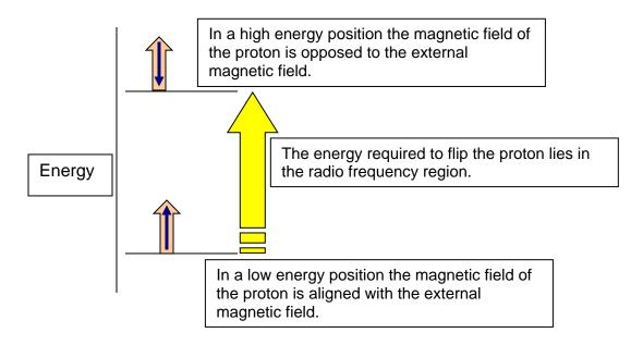
The actual energy required depends upon the exact environment on the proton. In nuclear magnetic resonance, **NMR**, spectroscopy a substance is placed in a strong magnetic field and subjected to a range of radio frequencies. The point at which a particular radio frequency is absorbed will depend upon the environments of the protons present in that substance.
