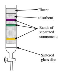
If the component is coloured, it is clear when it emerged from the column. If can be collected and the solvent evaporated to obtain the pure substance. If the substance is colourless, there are other ways of detecting their presence, for example certain materials glow in ultra-violet light.
