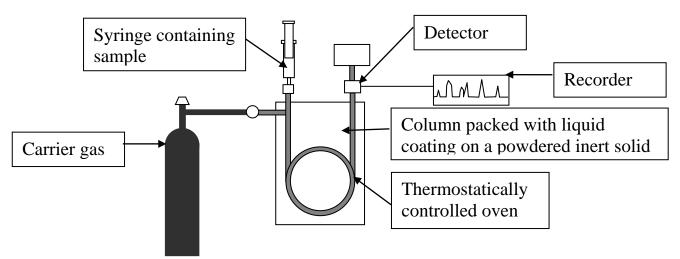
The vaporized sample is injected into the carrier gas which moves through the tube at a constant rate. Volatile components of a mixture are carried through the tube fast, while those that are more soluble in the mobile phase take longer to pass through the tube. The time a component spends going through the tube is called the **retention time**.
