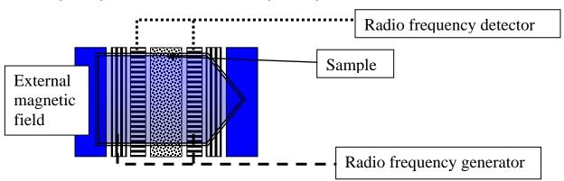
The detector will show which radio frequencies are absorbed. The system is calibrated, usually using the compound **tetramethylsilane**, **Si(CH<sub>3</sub>)<sub>4</sub>**, as the 0 point and then other frequencies compared to this as shift values.
